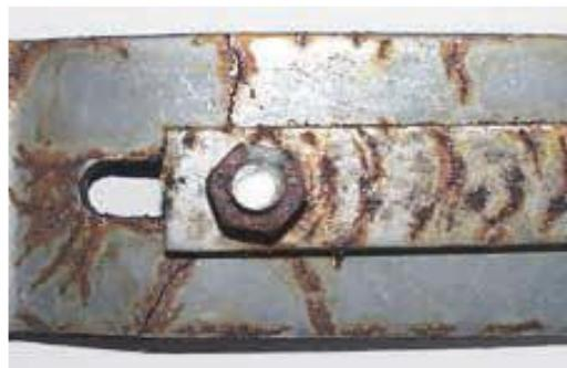
**Gambar 2.12** Korosi Tegangan
