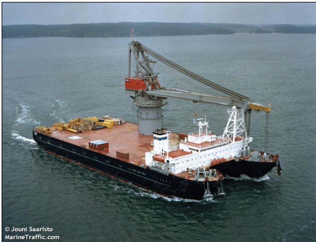
Gambar 1.1 Floating crane catamaran (Marine Traffic.com)
