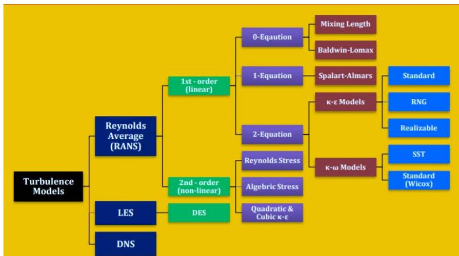
Gambar 2-10 Model Turbulensi
