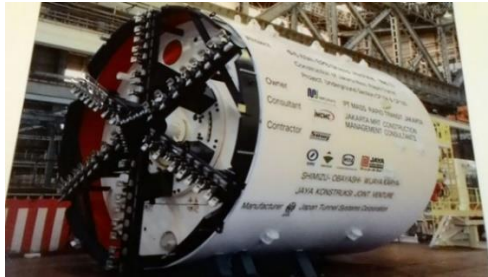
Gambar 2. 4. TBM Proyek MRT
