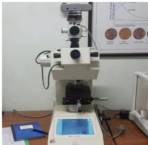
**Gambar 3. 4** Mesin Micro Vickers Hardness
