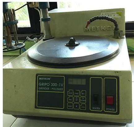
**Gambar 3. 3 Mesin Metkon Gripo 300-IV Grinder & Polisher**
