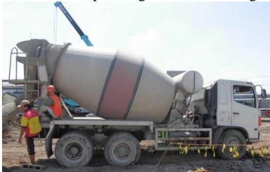
Gambar 2. 23 Truck Mixer Beton
