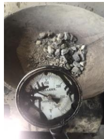
5. Cek suhu Agregat, pastikan suhu minimal 150C
