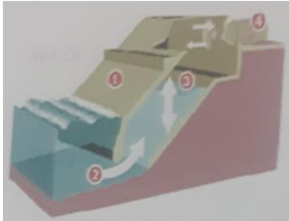
Gambar 2. 25 Penampang OWC tipe fixed. [10]
