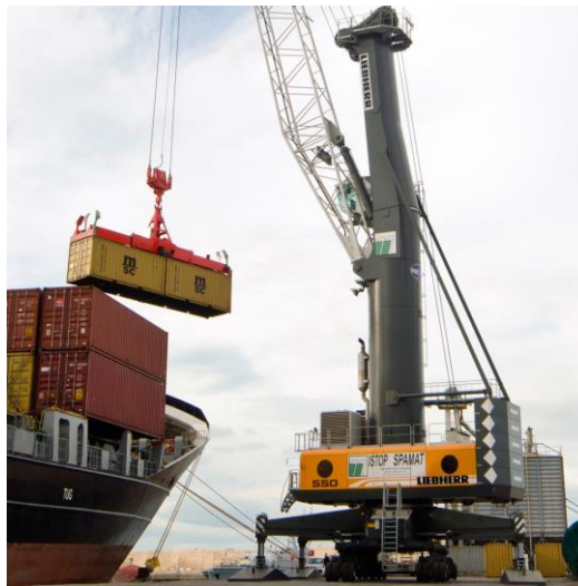
Gambar 2-3 Harbour Mobile Crane (HMC)
