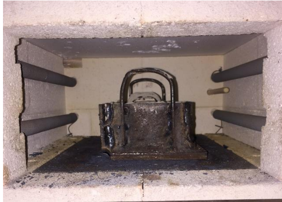
Figure 3.8 Reaction Pack in the Furnace
