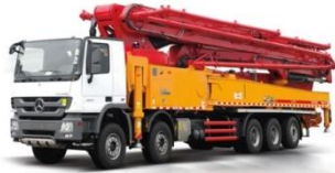
Gambar 2. 9 Concrete Pump Truck
