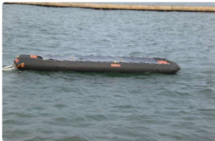
Gambar 2.6 *Floating Oil Storage*. (Slikbar, Slikbar.co, 2020)
