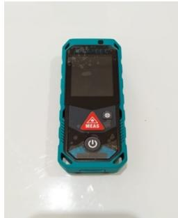
Gambar 3.5 *Laser Distance Meter*
