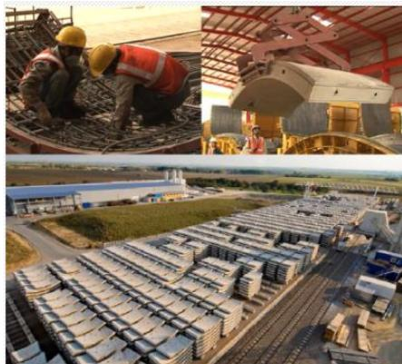
Gambar II-8 *Lining Precast* MRT
