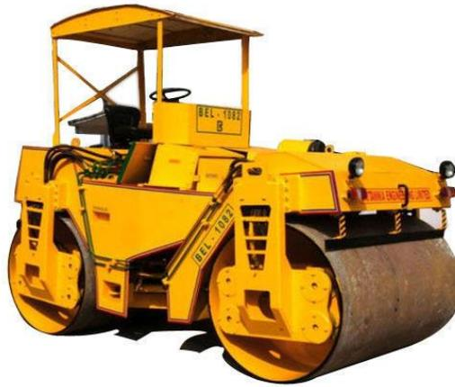
**Gambar 2.2 *Vibration Roller***
