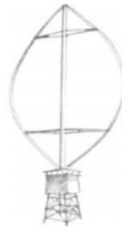
Gambar 2.7 Turbin Angin Darrieus VAWT Tipe Eggbeater (atau Curved Bladed ) (Rahmat Taufiqqurahman, 2016)
