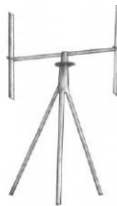
Gambar 2.16 Turbin Angin Darrieus VAWT Tipe H-Rotor (Rahmat Taufiqqurahman, 2016)
