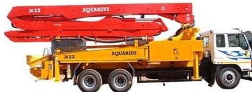
**Gambar 2. 10 Concrete Pump**
