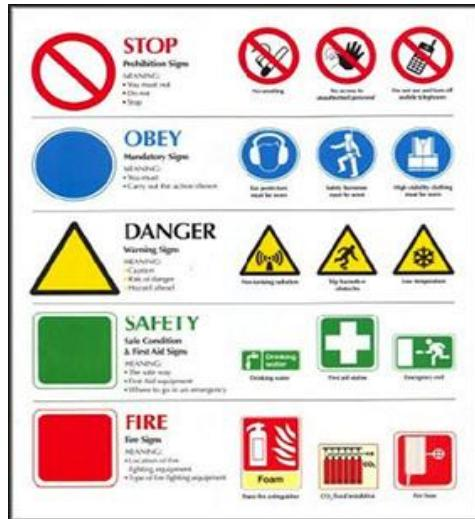
Gambar 2. 20 Rambu-Rambu K3
