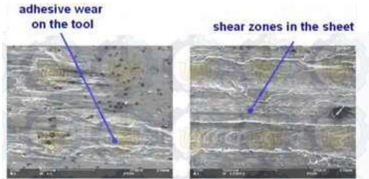
Gambar 2.8 Pengamatan Mikroskopik Adhesive Wear
