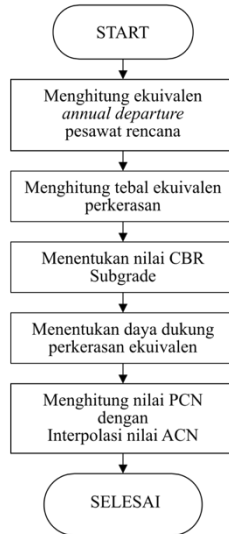
Gambar 3.7 Flowchart perhitungan PCN metode Klasik
