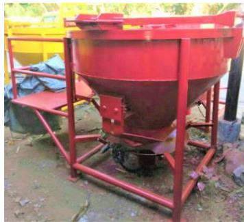
Gambar 2. 9 Concrete Bucket 1 m3
