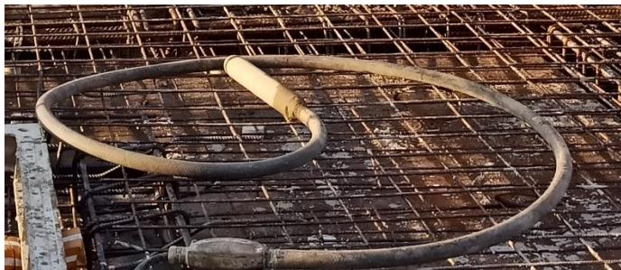
**Gambar 2.10 *Concrete Vibrator***
