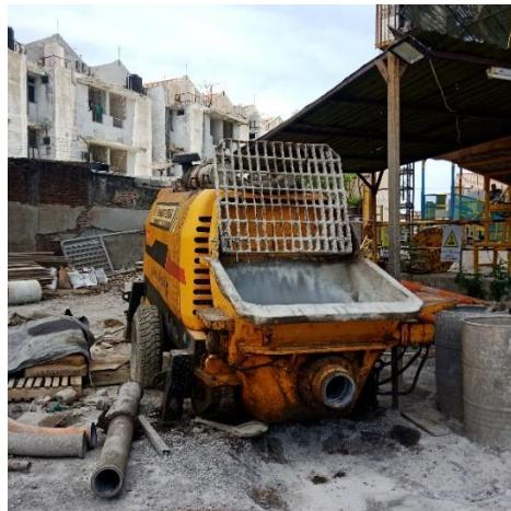
**Gambar 2.9 Concrete Pump**
