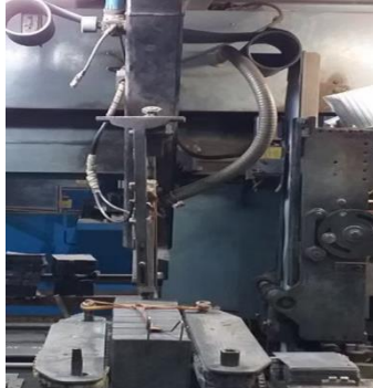
Gambar 2. 7 Separator Insertion System
