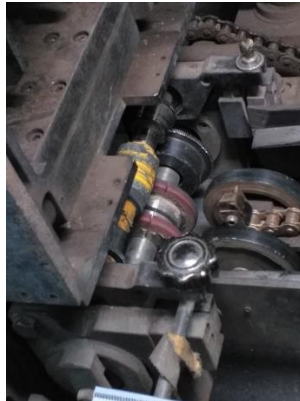
Gambar 4. 21 roll welding station
