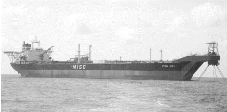
Gambar 2. 10. Konfigurasi Turret Mooring System (TMS)
