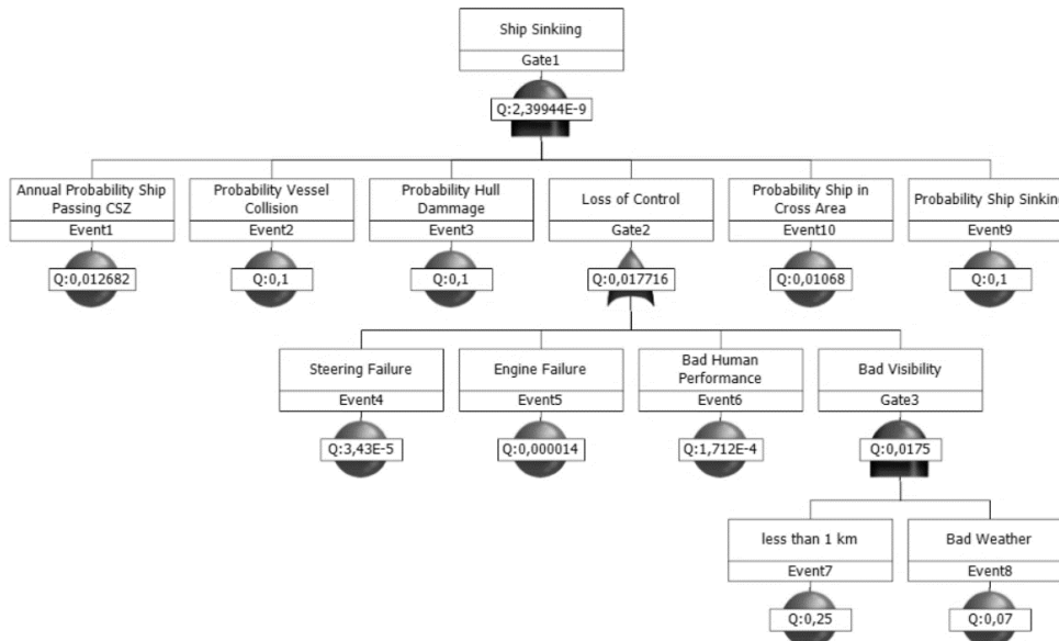
Gambar 4. 6. Contoh Hasil FTA Ship Sinking Skenario 2
