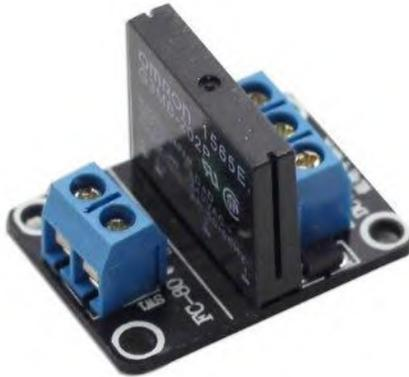
**Gambar 2.6** *Solid State Relay (SSR)*
