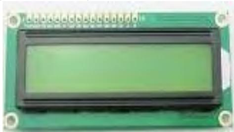
**Gambar 2.4** LCD 16X2
