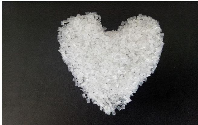
**Gambar 2.4** *Maleic-Anhydride Polypropylene* (MAPP)
