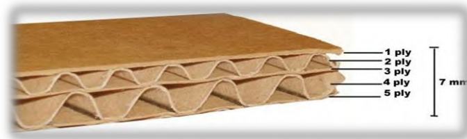
Gambar II. 15. Double wall corrugated fiberboard.
