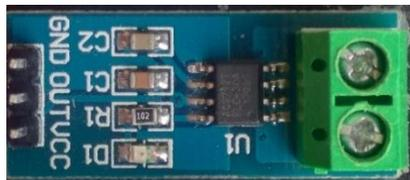
**Gambar 2.5.** Modul sensor arus ACS712
