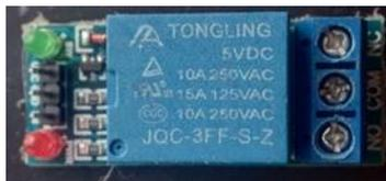
**Gambar 2.10.** Modul Relay 1 Channel 5VDC-220VAC
