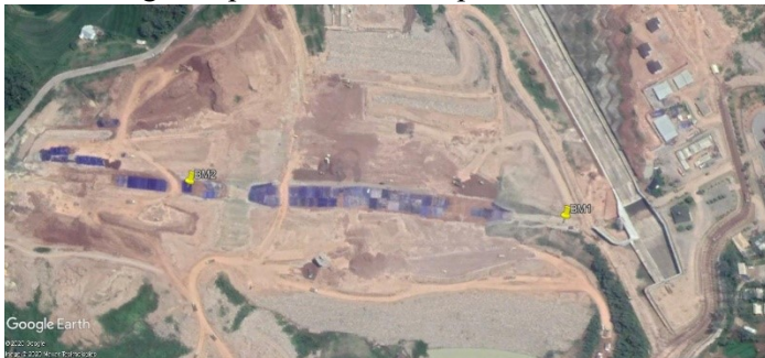
Gambar 4.2 Titik BM As Tubuh Bendungan
