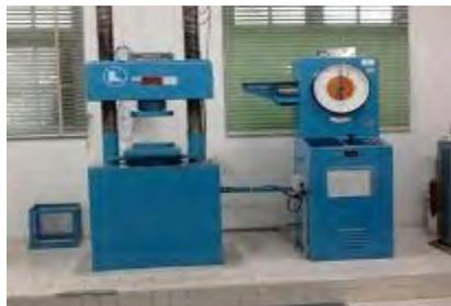
Gambar 2.4 Toorse universal testing machine
