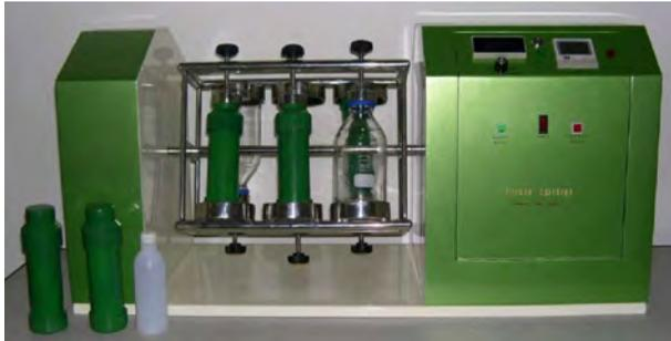
Gambar 2.5 Rotary agitator model SO192
