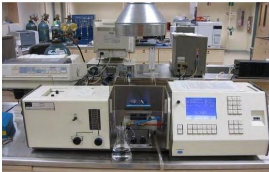
Gambar 2.6 Atomic absorption spectrophotometer
