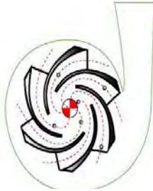
**Gambar 2.1 Pompa Sentrifugal**
