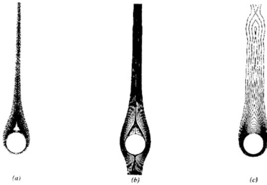
Gambar 2.11. Vortex shedding disekitar heated cylinder dengan  $Re=100$ ,  $Ri=1.0$  : a). streaklines, b). streamlines, c). isotherms (Hatanaka et al, 1995)
