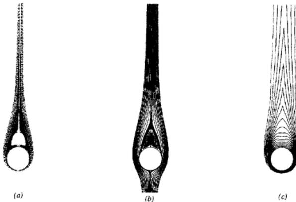
Gambar 2.10. Vortex shedding disekitar heated cylinder dengan  $Re=100$ ,  $Ri=0.5$  : a). streaklines, b). streamlines, c). isotherms (Hatanaka et al, 1995)
