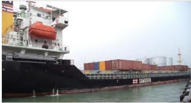
Gambar 2.6 SPCB (*Self Propelled Container Barge*)
