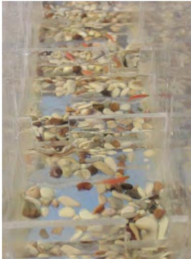
**Gambar 4.7.** Model test hidrolika fishway berskala
