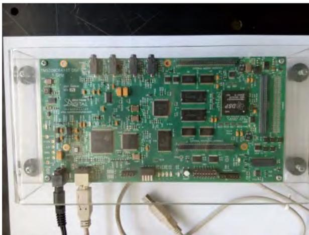
**Gambar 3.32** Gambar DSK TMS320C6416
