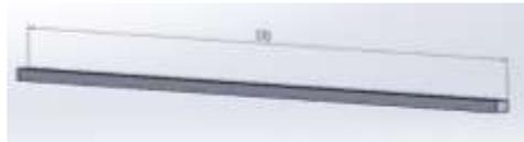
**Gambar 5.7** Hollow stainless steel 170 cm
