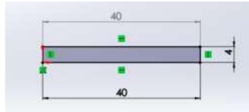
**Gambar 6.6** 2Dimensi Hollow stainless steel 40 cm
