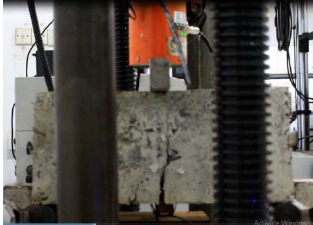
Gambar 3.7 Pengujian three Bending Point
