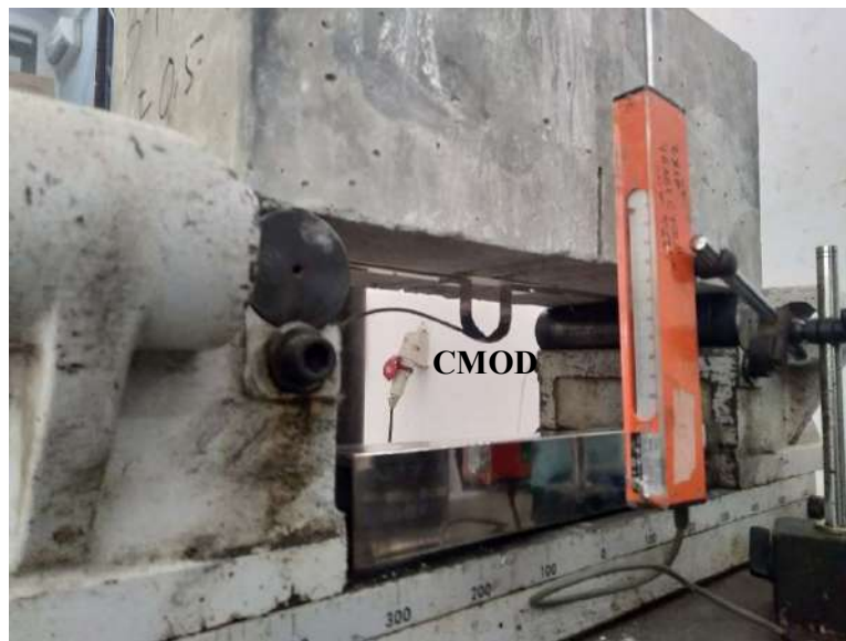
Gambar 3. 9 Crack mouth opening displacement (CMOD)
