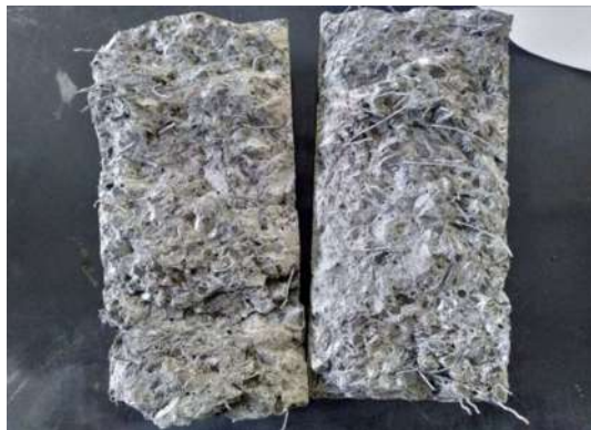
Gambar 4.5 Hasil pengujian splitting test
