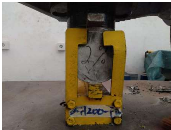
Gambar 3. 2 Hasil pengujian splitting silinder
