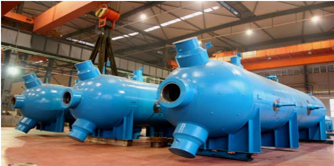
Gambar 2.8. High Pressure Heater [6].
