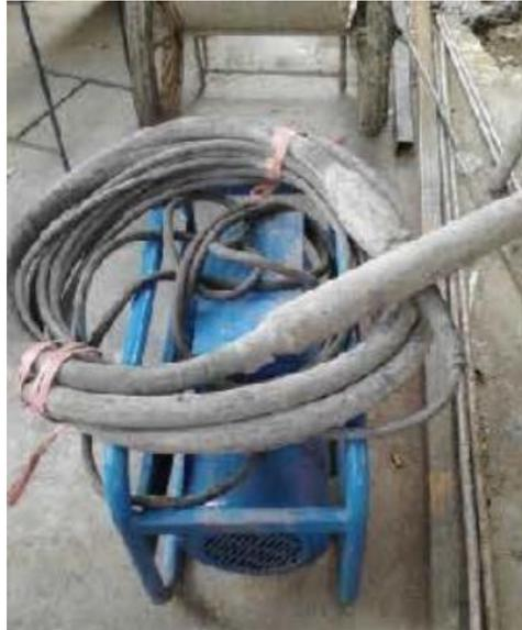
**Gambar 3. 13 Concrete Vibrator**
