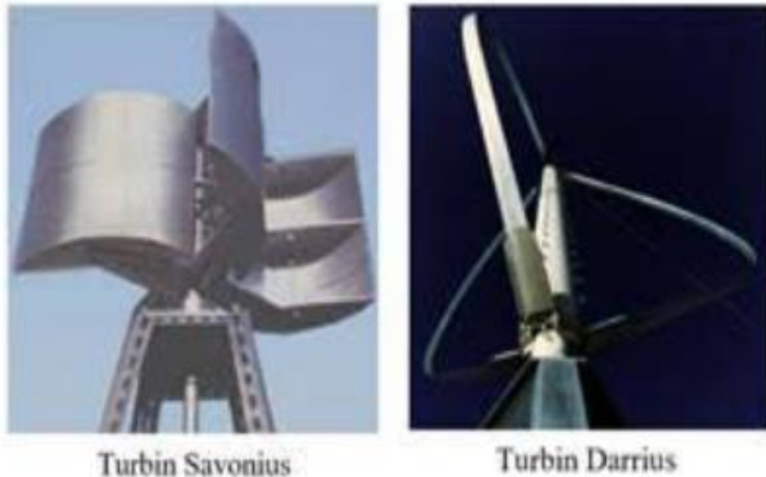
Gambar 2. 3 Tipe Turbin Angin VAWT (Hau 2006, 2010)
