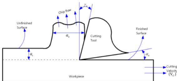
Gambar 2.26 Positive rake angle
