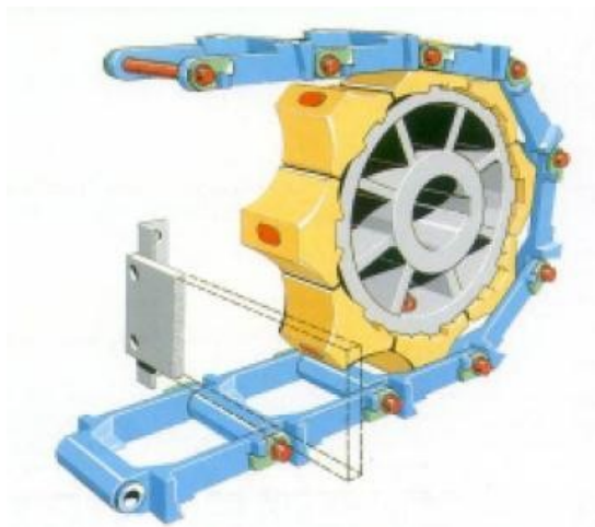
Gambar 5.2 Chain Drag Conveyor
