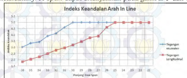
Gambar 4. Indeks Keandalan Free span arah In line
