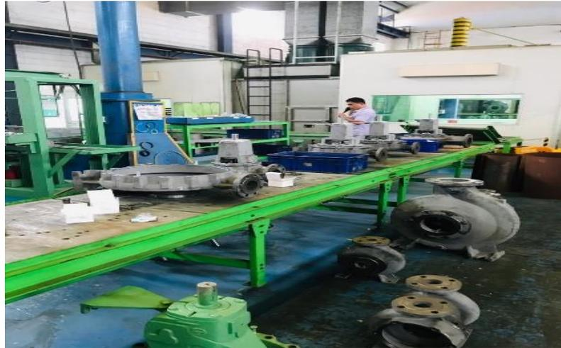
Gambar 1. 18 Assembly Pompa End Suction
