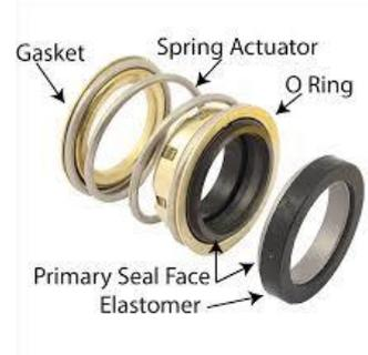
Gambar 2. 7 Mechanical Seal
