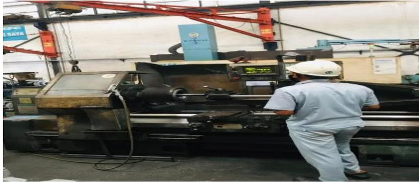
Gambar 1. 14 Proses Turning/Bubut
