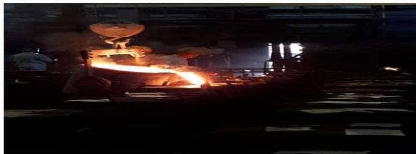
Gambar 1. 9 Proses Pouring Pada Molding
