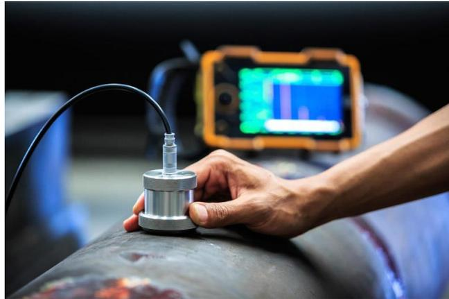
Gambar 2.5 *Ultrasonic Test*
