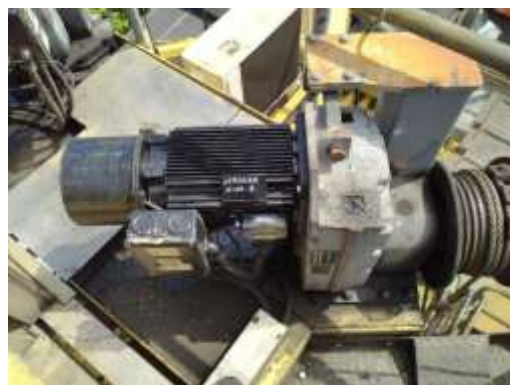
Gambar 2.14 ACM gear RTG
