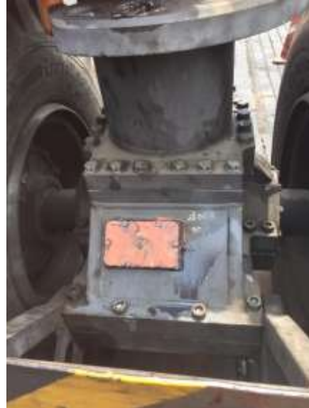
Gambar 2.21 Gantry gear travelling RTG
