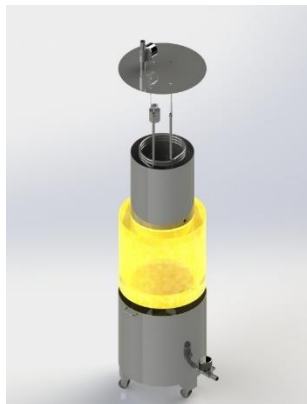
Gambar 4.36 Breakdown Part of Water Heater Heater Electric
