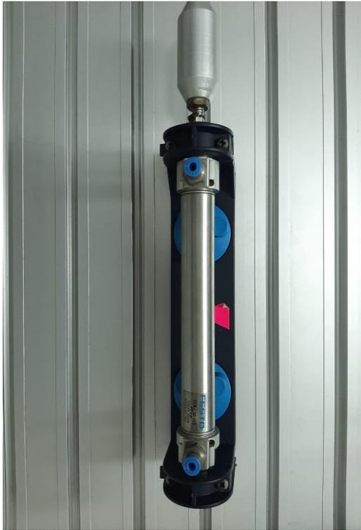
*Figure Double Acting Cylinder*
