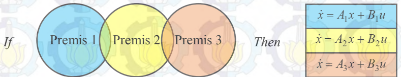
Gambar 2.7 Skema Parallel Distributed Compensation (PDC) [9]
