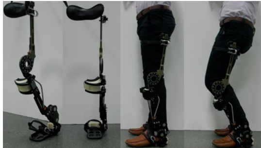
Gambar 2.9: Smart assistive posture device dengan human-chair system [8].
