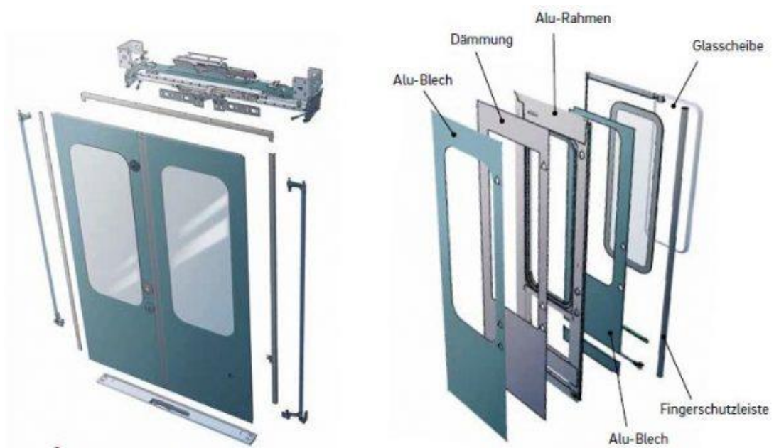
Gambar 4.43 Sliding Plug Door Component Sumber : railssystem.net
